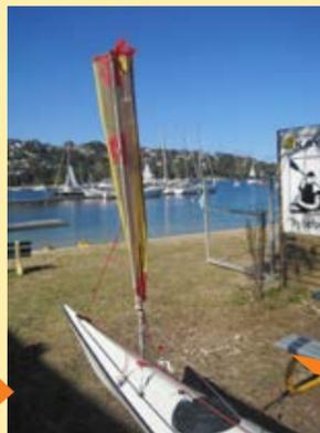
Then move the retractable dog lead switch to 'retract' and pull the boom down into the sailing position by means of the mainsheet. Switch RDL back to 'stop'. Sail away.
